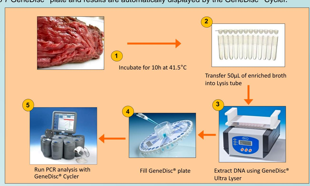
Figure 1: Workflow of the GeneDisc® STEC Top7 method.
