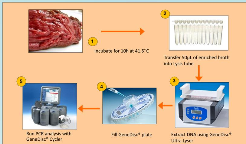
Figure 1: Workflow of the GeneDisc® STEC Top7 method.
